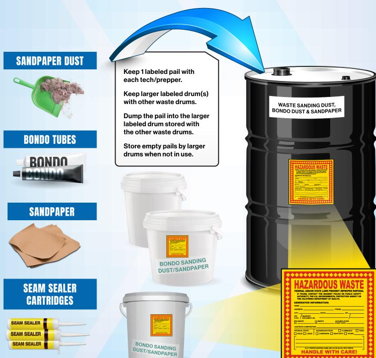
SUBMIT SERVICE CHANNEL WORK ORDER WHEN WASTE DRUM REACHES 75% FILLED AND/OR EXCEEDS ACCUMULATION OF 180 DAYS ON SITE.
